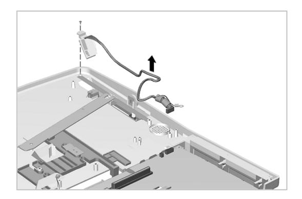
Figure 7-28. Removing the Power Switch Assembly
